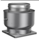
The CUBE is an aluminum exhaust fan specifically designed for roof or sidewall mounted applications where contaminated or grease laden exhaust air can be discharged directly upward, away from the roof or wall surface. The fans feature a one piece windband continuously welded to curb cap and double studded isolators for true vibration isolation.
