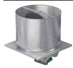
Model RBU is an upblast axial exhaust fan designed to discharge air and contaminants up and away from the roof deck for commercial and industrial applications like warehouses, manufacturing facilities and distribution centers. Utilizing a welded steel propeller, this belt-driven fan is designed to run at lower RPMs, producing lower sound levels and is recommended for sound sensitive applications. The motor is located inside of the airstream and is cooled as air exhausts over the motor.
