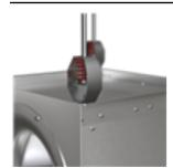
Complete hanging isolation kit with spring isolators to reduce vibration and sound levels. Support brackets included are designed to permit mounting of the fan with the motor located on top, bottom or side. Includes Brackets, Springs, Isolator Cap, Isolator Hanger & Washer, IOM, and Hardware.
