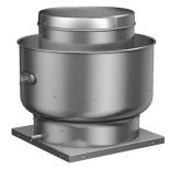
Model CUE is a direct drive exhaust fan specifically designed for roof or sidewall mounted applications discharging the air directly upward, away from the roof or wall surface. The fans feature a one piece windband continuously welded to curb cap and double studded isolators for true vibration isolation.
