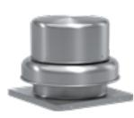
Model GB, belt drive centrifugal roof exhaust fans are designed to meet the general clean air exhaust requirements for industrial and commercial buildings. Units feature a fully rolled windband bead for increased stability and easy transport. Fresh outside air is drawn in under the motor cover to maximize motor life.
